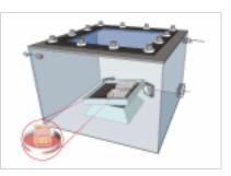
IPREM researchers have developed a system in which skin cells and biopsies can be exposed to a mixture of volatile organic compounds representative of indoor air pollution.
